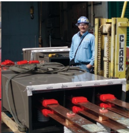
63kA short circuit KEMA design testing
