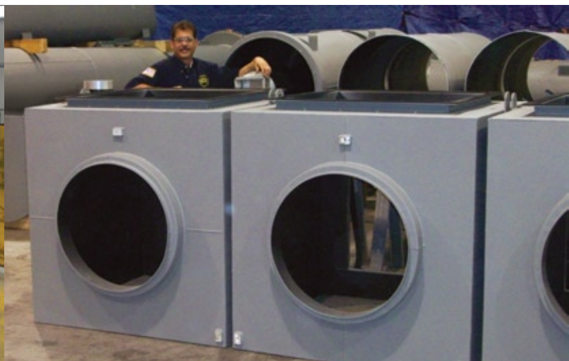
Transformer low voltage bushing enclosures
